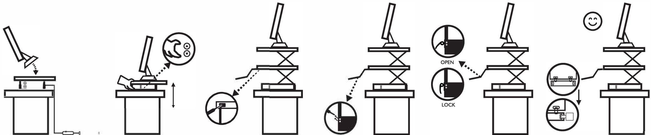
1. Place **CHANGEdesk** on top of any level desk, table, or counter. Connect one end of the power cord to **CHANGEdesk** and the other end to an electrical outlet.
